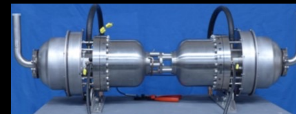
1.8 kWe generator: Two 1 kWe Stirling converters mounted dual-opposed (Army Research Lab)
